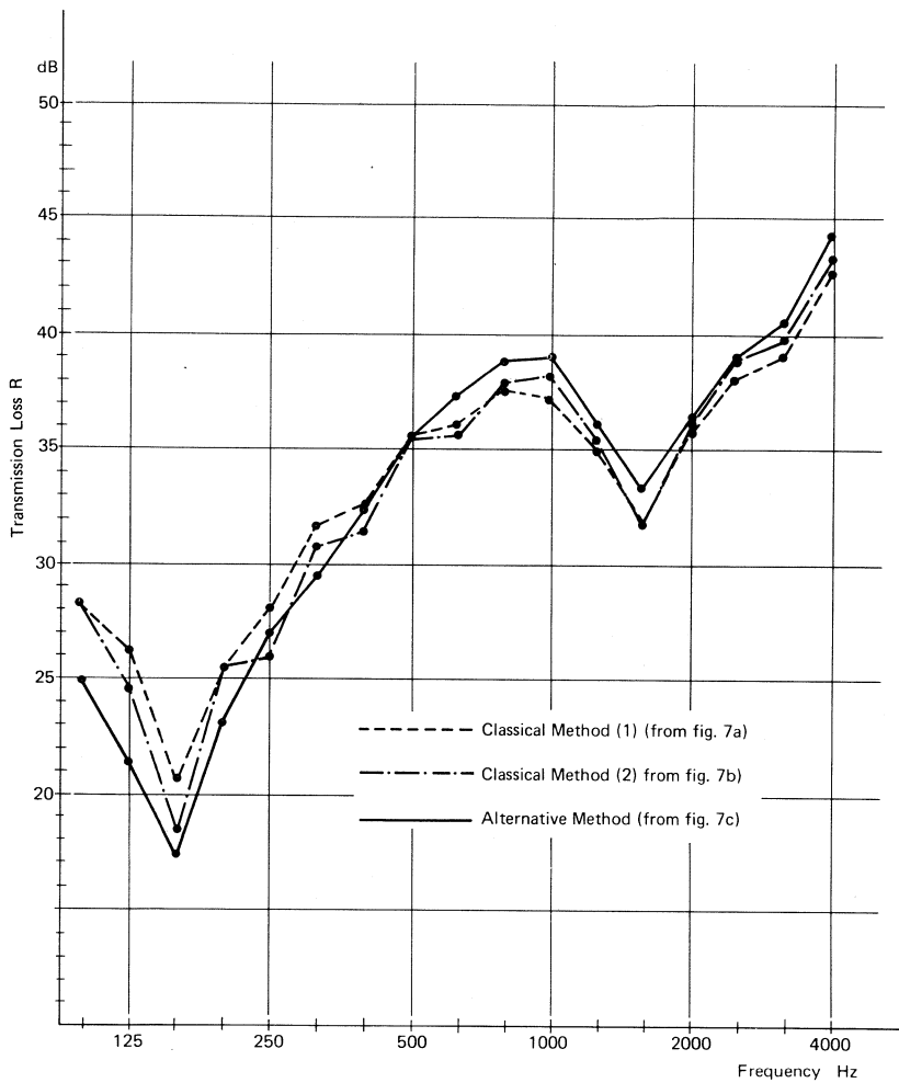
Fig.8. Transmission loss mean values of both directions obtained from Fig.7 for the three methods
